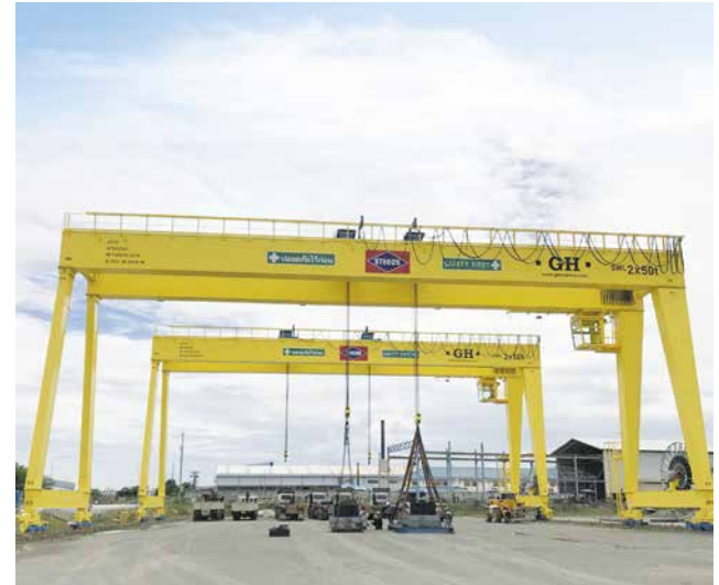
Mobile cranes with double beam of 100 t. (above) and 22 t. (below), in two STECON projects in Thailand.
